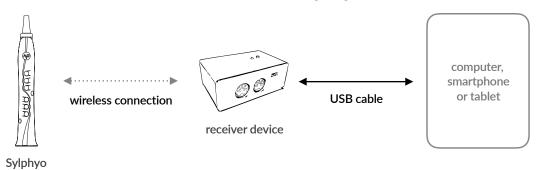
The receiver device should be recognized by your operating system as a standard USB MIDI device.
