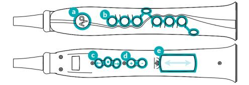
a The Aodyo key (^P) allows you to enter Quick settings, which you enter as soon as the key is pressed, and leave as soon as it is released.
