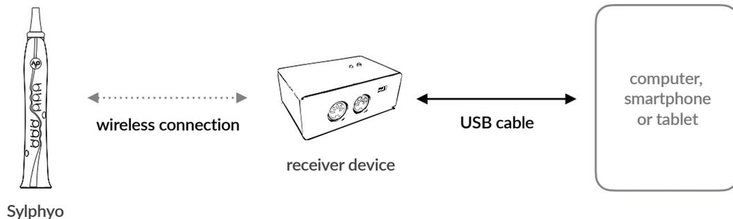
The receiver device should be recognized by your operating system as a standard USB MIDI device.
