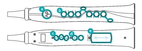
a The Aodyo key ( $^{\circ}$ ) allows you to enter Quick settings, which you enter as soon as the key is pressed, and leave as soon as it is released.
