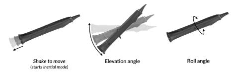
Now, slowly **tilt** your Sylphyo from the vertical to the horizontal position. You should start hearing sound at a 45° angle, and it should reach its maximum intensity when the Sylphyo is horizontal. In inertial mode, the *elevation angle* of your Sylphyo always replaces the intensity of your breath in the control of sounds.
