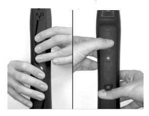
First, **touch** all the note keys except the one under your left little finger, simultaneously with the middle *octave key* on the back of your Sylphyo. When blowing into the mouthpiece, you will play a *C* note on the third octave<sup>1</sup> (*C3*).
