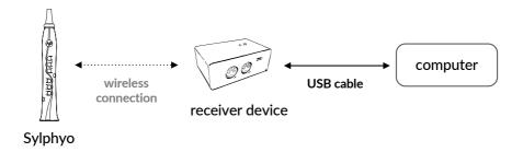
The receiver device is immediately recognized as a standard USB-MIDI peripheral, thus no drivers are required.
