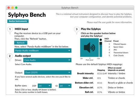
First, select **Panda-Audio midiBeam** as a **MIDI input**, assuming the receiver device is already plugged in. Else, plug it to a USB port on your computer, and hit the **Refresh** button before selecting the MIDI input again.
