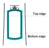
To control more parameters, you can also have the slider perform a different function depending on whether you start touching it on the *Top*
