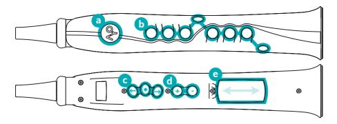
a The Aodyo key (^P) allows you to enter Quick settings, which you enter as soon as the key is pressed, and leave as soon as it is released.
